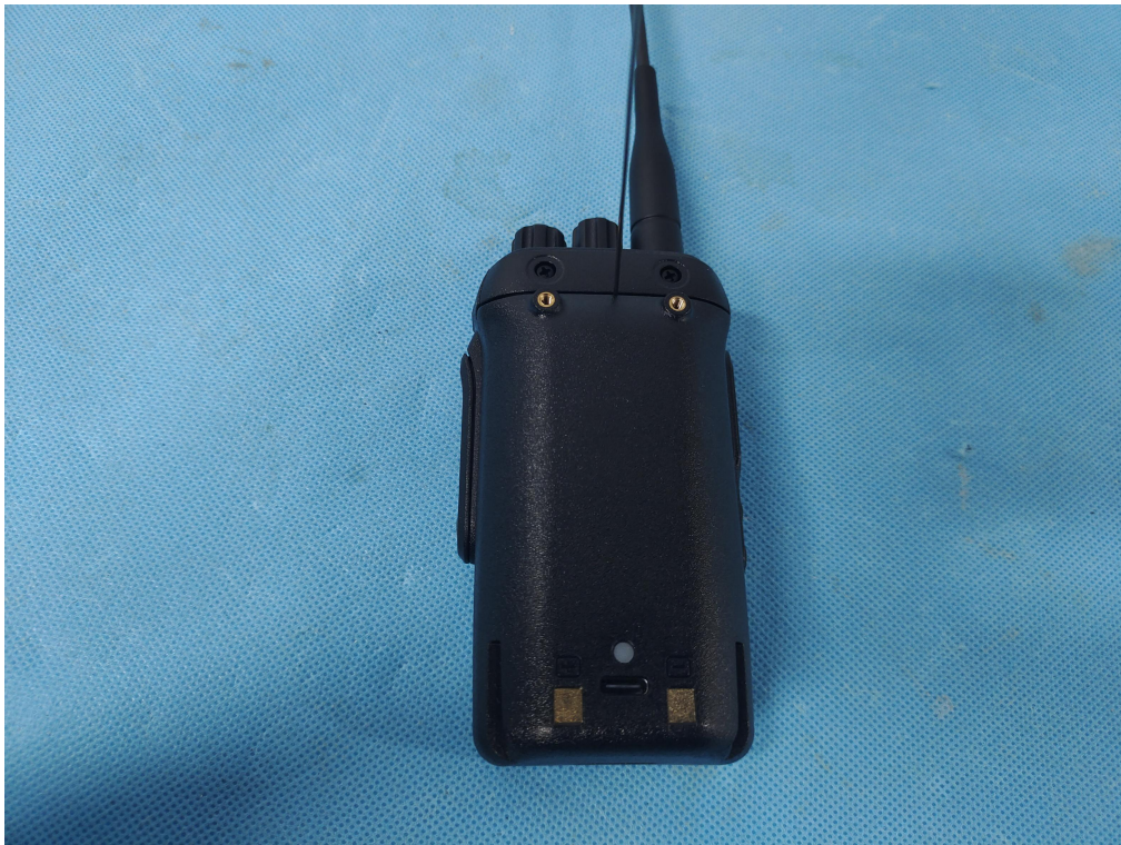
Fig.5 – view after testing (IP6X)
