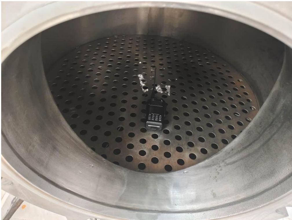
Fig.3 – view during testing (IPX8)
