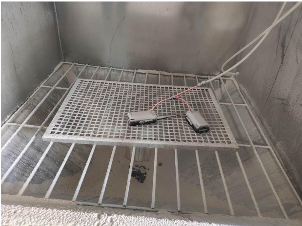
Fig.6 – view after testing (IP6X)
