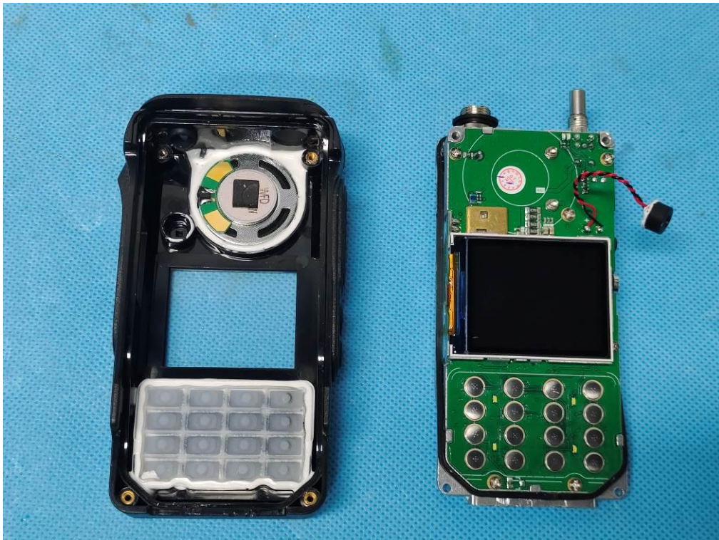
Fig.7 – view after testing (IP6X)
