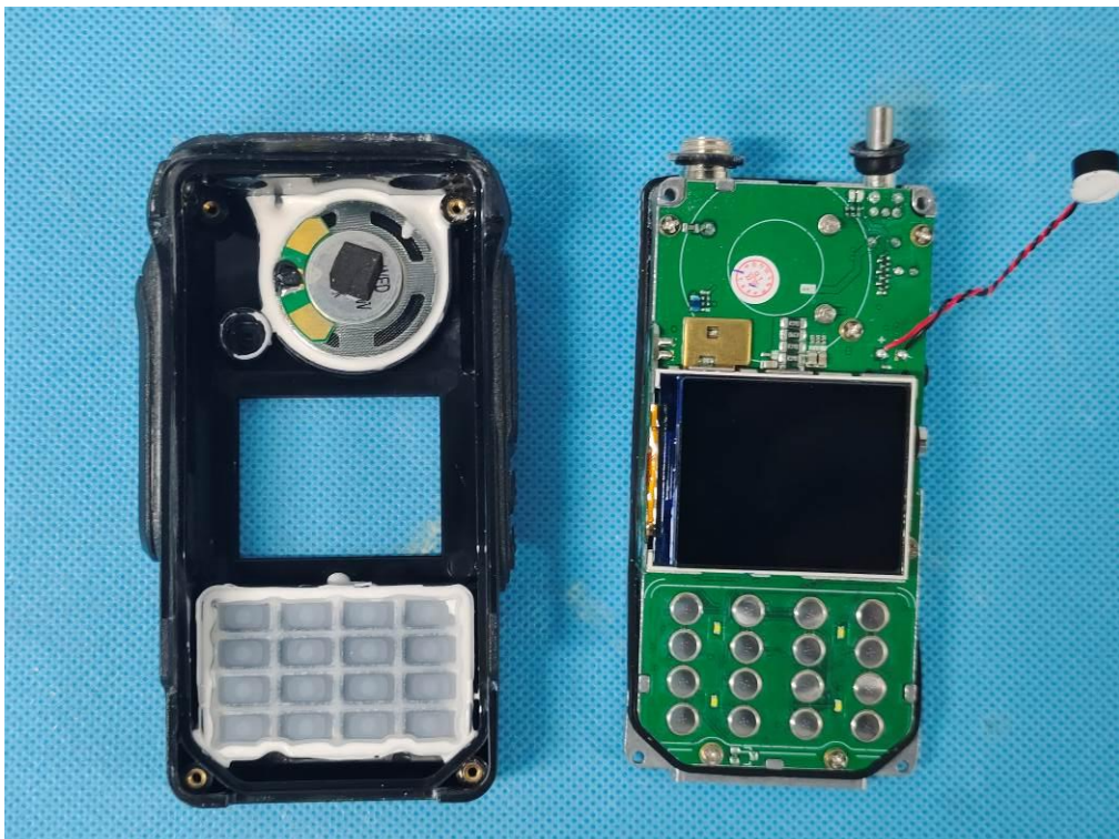
Fig.4 – view after testing (IPX8)
